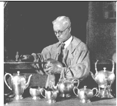
Figure 9 Using a Snarling Iron
